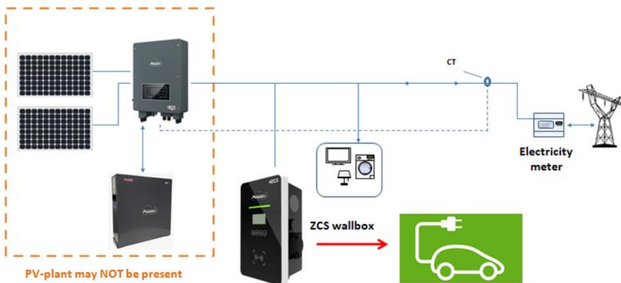
Figure 3 – Example of a charging station connected to a PV system (optional) and grid
