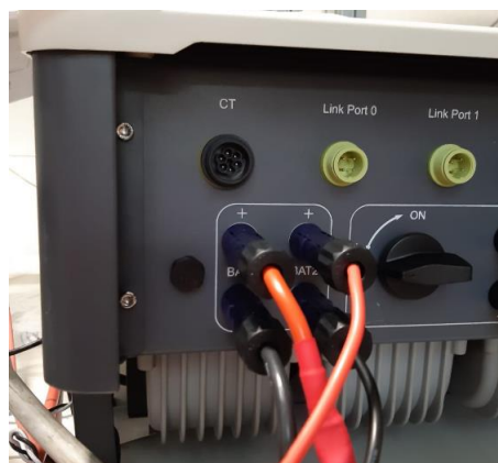
Figure 31 - Inverter-side DC power connection with two battery inputs populated
