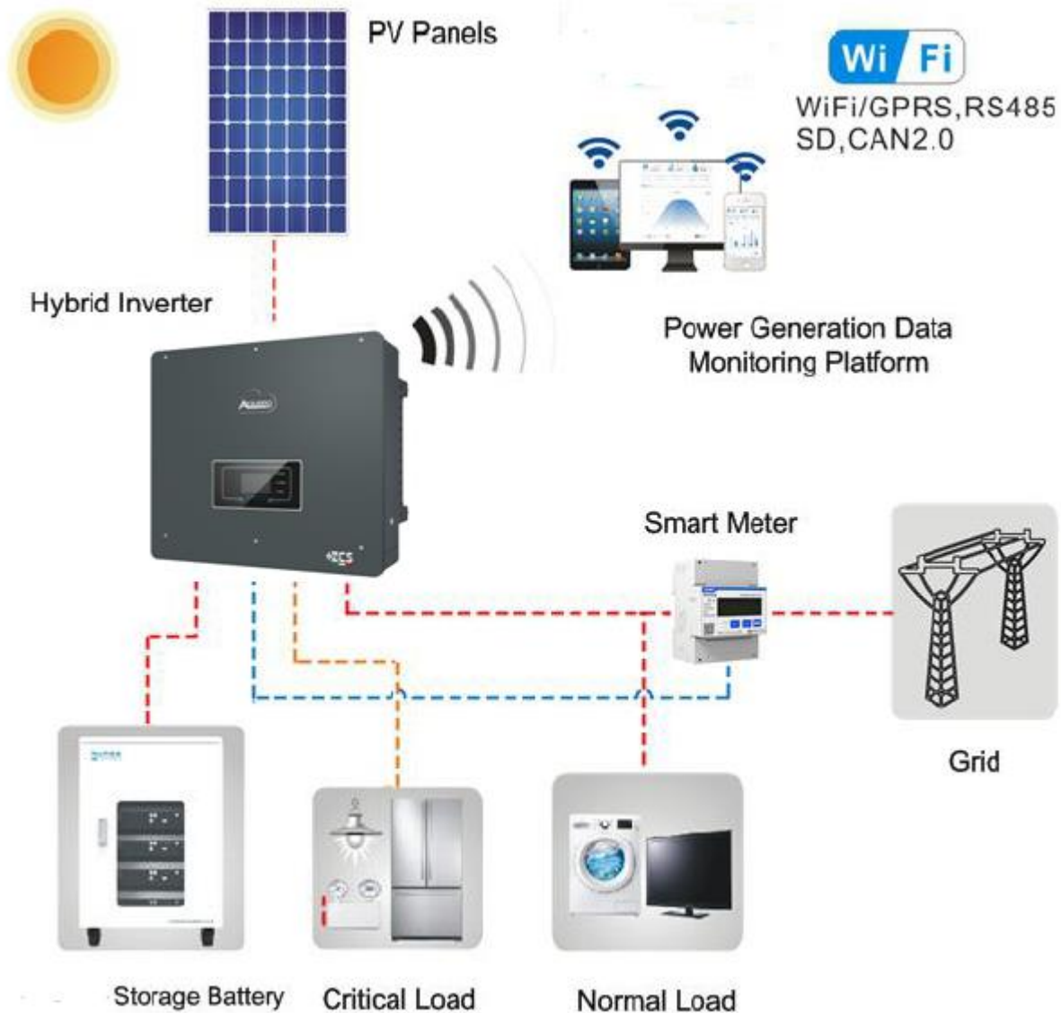
Figure 1 - Diagram of a system with 3PH HYD5000-HYD20000-ZSS hybrid inverter
