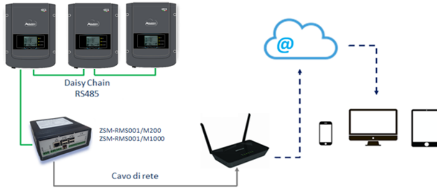
Figure138- Diagram showing the operation of the ZSM-RMS001/M200 / ZSM-RMS001/M1000 datalogger
