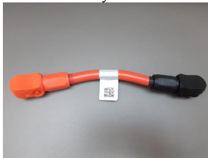
Figure 17 - Power connector between battery modules
