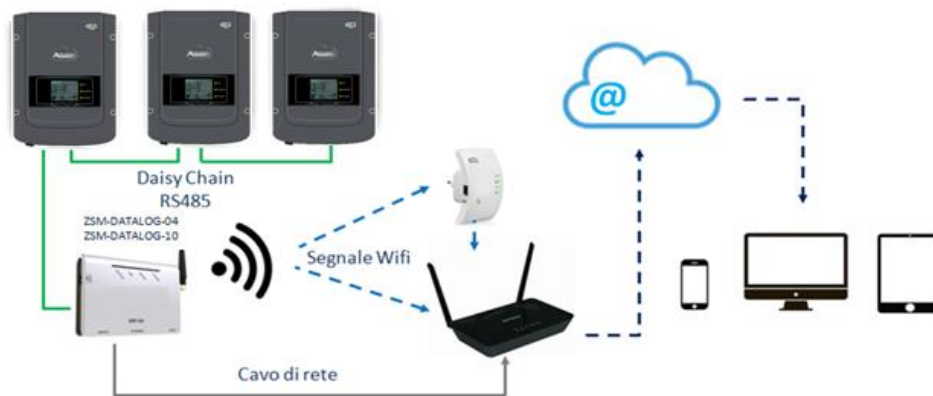
Figure 137 – Diagram for connecting the ZSM-DATALOG-04 / ZSM-DATALOG-10 datalogger
