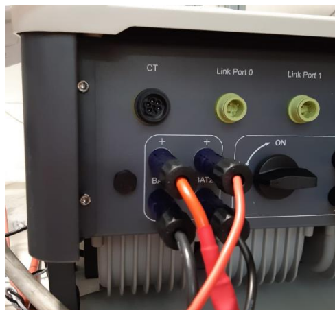
Figure 41 - Inverter-side DC power connection with two battery inputs populated
