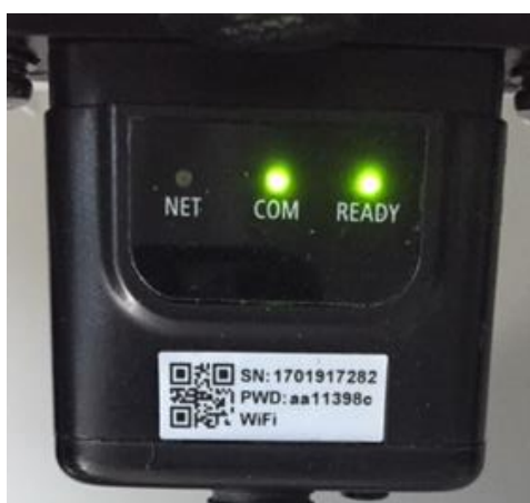
Figure 57 - Irregular communication status between Wi-Fi and remote server
