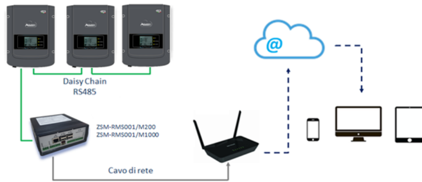
Figure 75 - Diagram showing the operation of the ZSM-RMS001/M200 / ZSM-RMS001/M1000 datalogger
