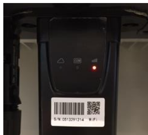
Figure 57 - Irregular communication status between Wi-Fi and remote server
