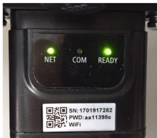
Figure 66 - Irregular communication status between the inverter and adapter
