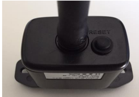
Figure 54 – Reset button on the Wi-Fi adapter
