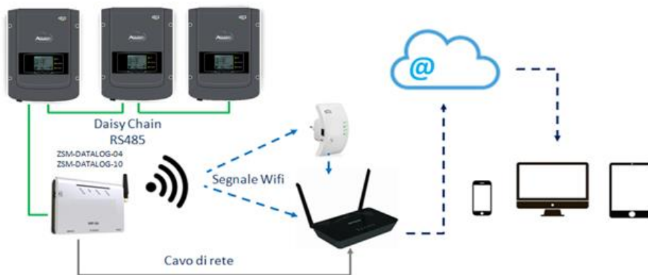
Figure 74 – Diagram for connecting the ZSM-DATALOG-04 / ZSM-DATALOG-10 datalogger
