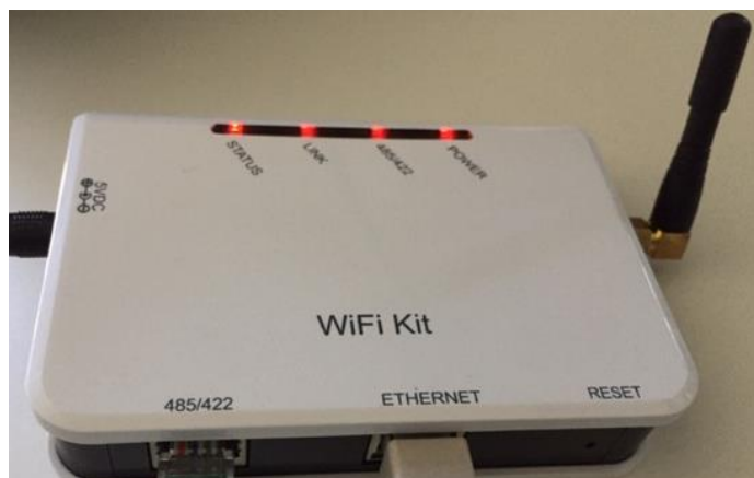
Figure 95 – LED indicating the correct configuration of the datalogger
