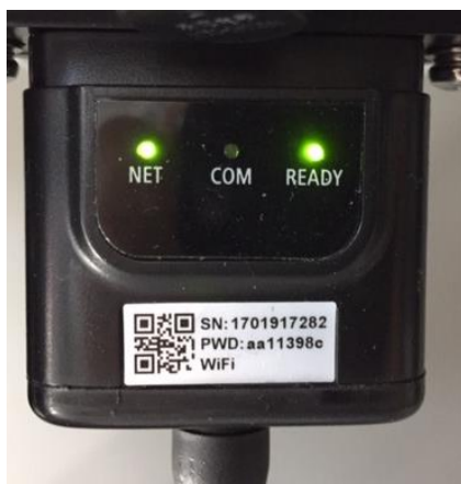
Figure 55 - Irregular communication status between inverter and Wi-Fi
