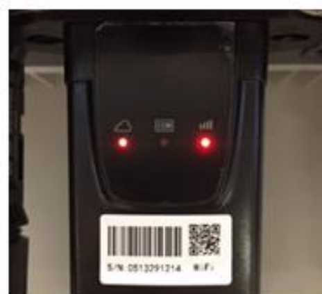
Figure 55 - Irregular communication status between inverter and Wi-Fi
