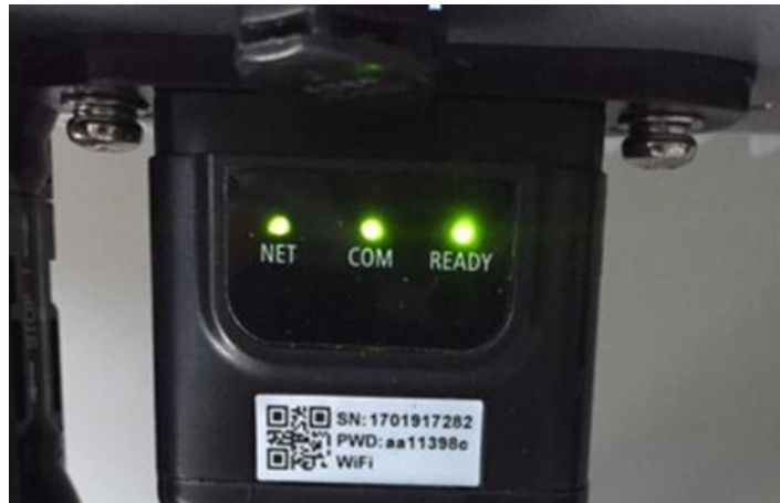
Figure 65 - Final status of LEDs
