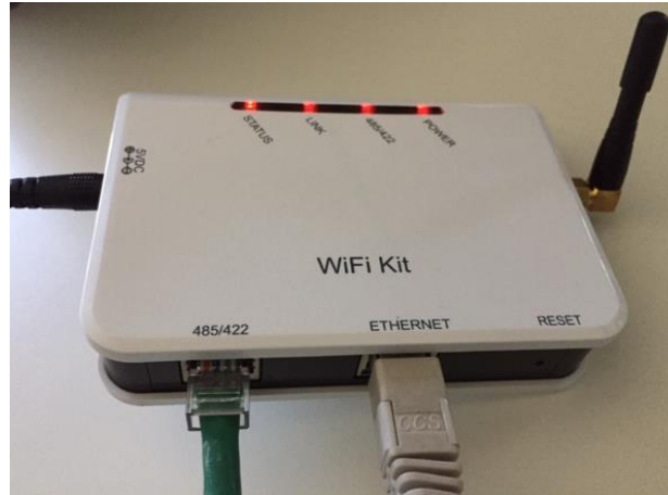
Figure 82 - Ethernet cable connected to the datalogger
