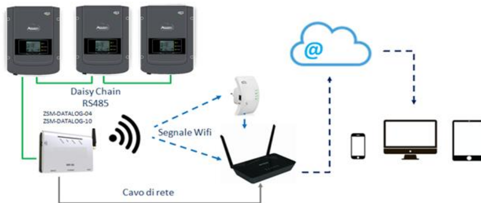
Figure 73 – Diagram for connecting the ZSM-DATALOG-04 / ZSM-DATALOG-10 datalogger
