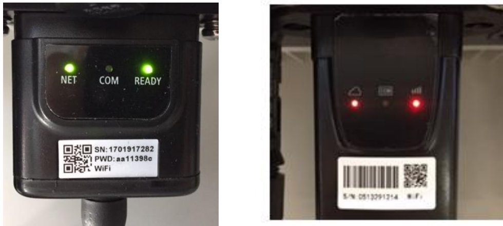
Figure 54 - Irregular communication status between inverter and Wi-Fi
