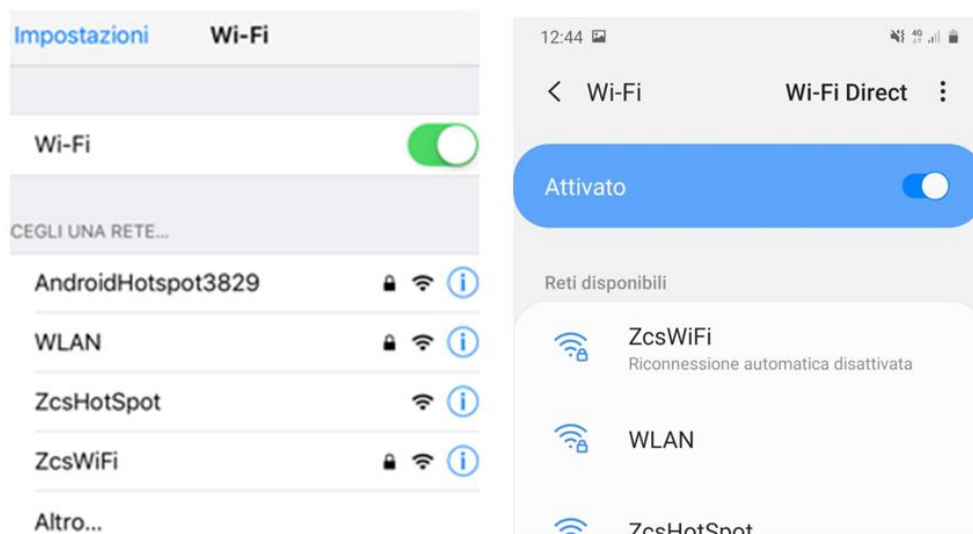
Figure 49 – Wi-Fi network search on Smartphone (iOS and Android); Access point of the Wi-Fi adapter is no longer visible
