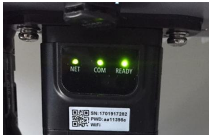
Figure 72 - Final status of LEDs
