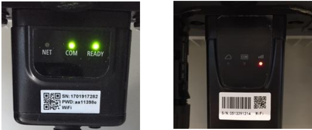
Figure 64 - Irregular communication status between Wi-Fi and remote server
