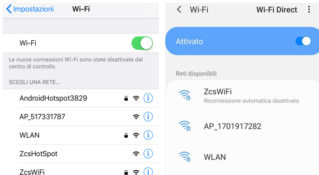
Figure 44 - Search for Wi-Fi networks on iOS smartphone (left) and Android smartphone (right)
