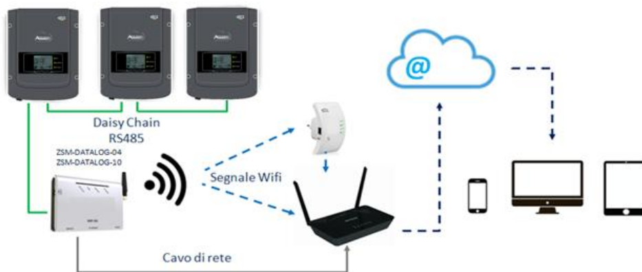
Figure 81 - Diagram for connecting the ZSM-DATALOG-04 / ZSM-DATALOG-10 datalogger
