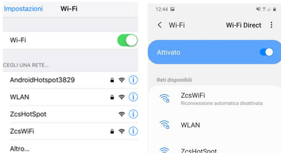
Figure 57 – Wi-Fi network search on Smartphone (iOS and Android); Access point of the Wi-Fi adapter is no longer visible
