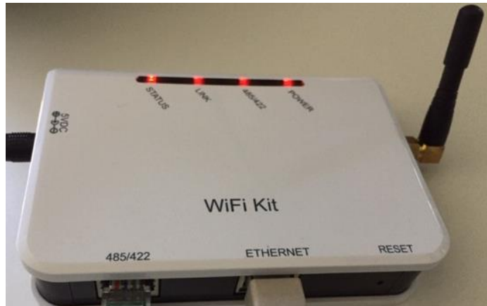
Figure 150 - LED indicating the correct configuration of the datalogger
