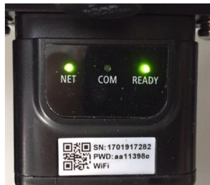
Figure 126 - Irregular communication status between inverter and adapter
