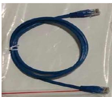
Figure 17 - Communication cable between WeCo 4k4 batteries
