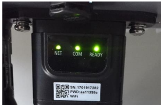
Figure 125 - Final status of LEDs
