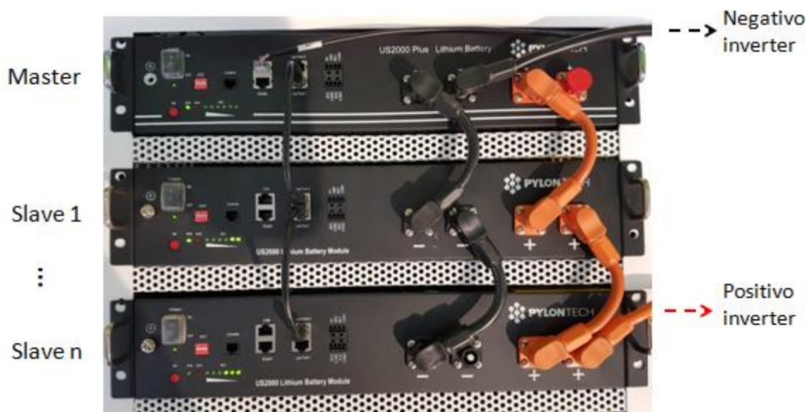
Figure 11 - Connecting three Pylontech batteries in parallel
