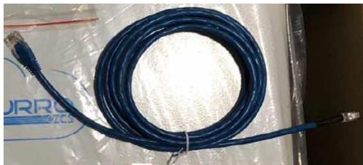
Figure 22 - Communication cable between the inverter and the WeCo PRO 4k4 battery
