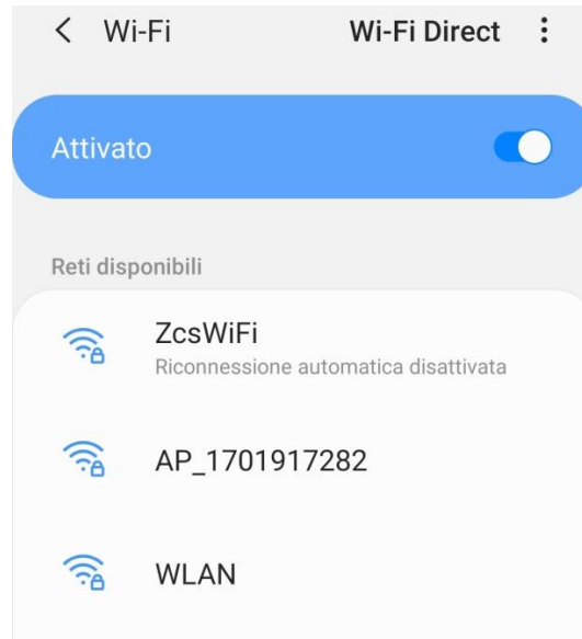
Figure 94 – Disabling automatic reconnection to a network
