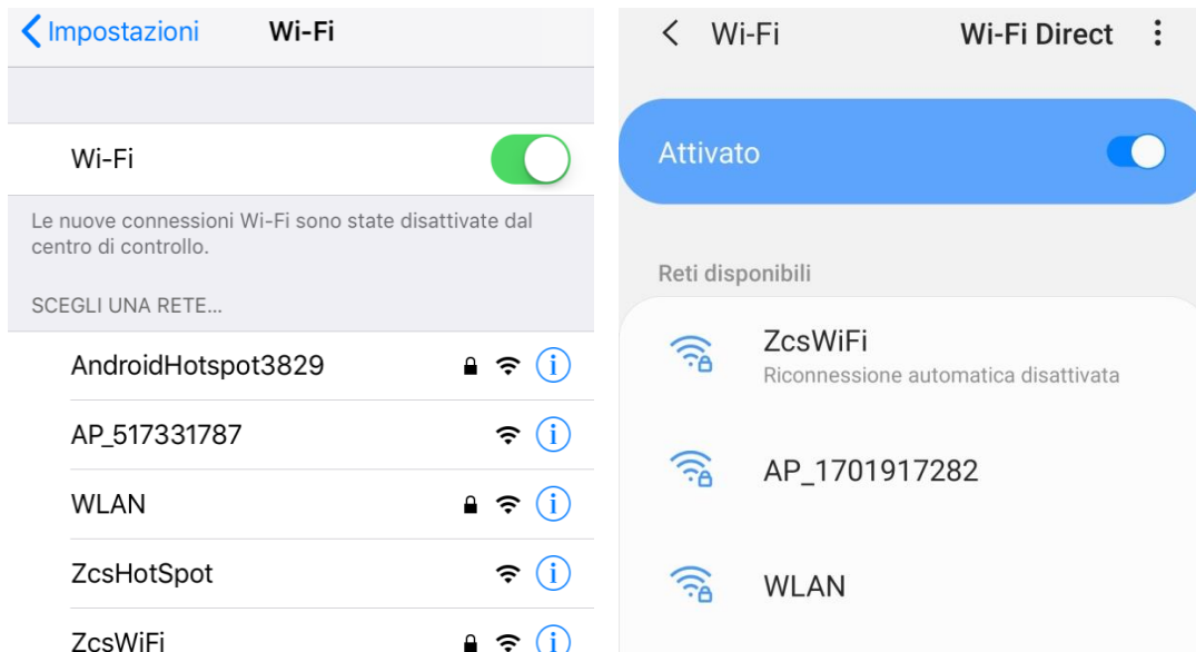
Figure 93 - Search for Wi-Fi networks on iOS smartphone (left) and Android smartphone (right)
