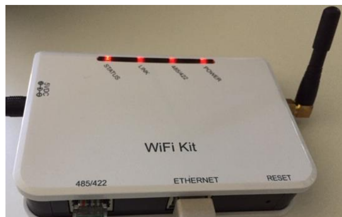
Figure 118 – LED indicating the correct configuration of the datalogger
