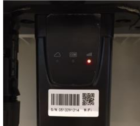
Figure 81 - Irregular communication status between Wi-Fi and remote server
