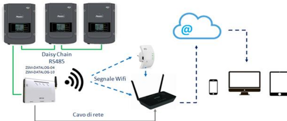
Figure 98 - Diagram for connecting the ZSM-DATALOG-04 / ZSM-DATALOG-10 datalogger
