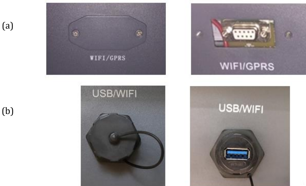
Figure 59 – Port for external Wi-Fi adapter
