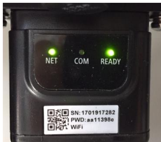
Figure 90 - Irregular communication status between the inverter and adapter
