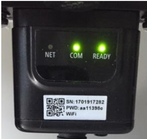
Figure 81 - Irregular communication status between Wi-Fi and remote server
