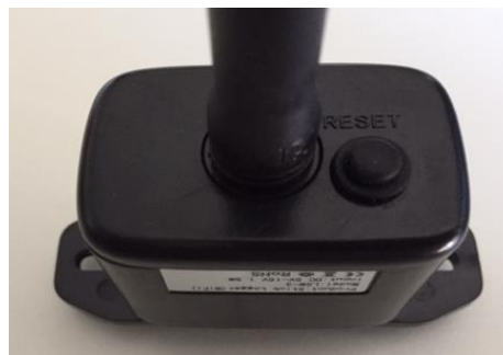
Figure 78 – Reset button on the Wi-Fi adapter
