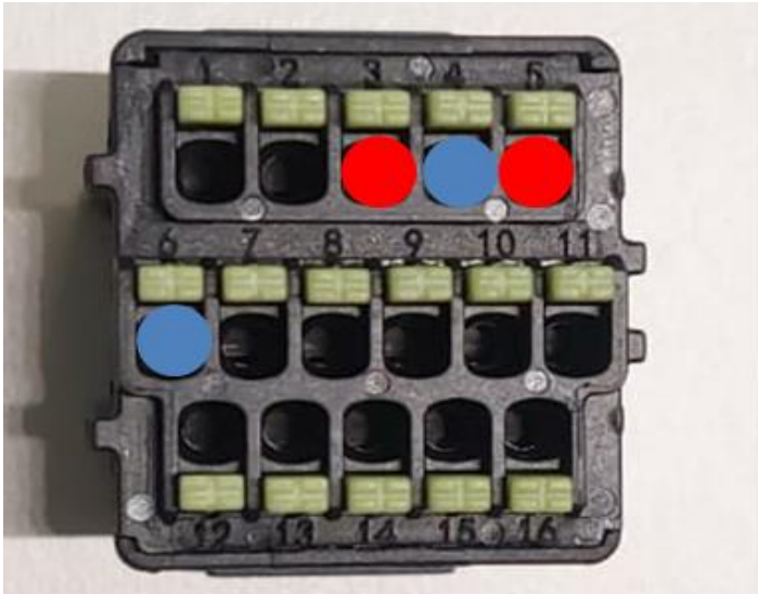
Figure 103c – Connecting the serial line via the communication connector for 1PH HYD3000-HYD6000-HP
