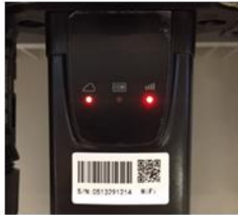
Figure 79 - Irregular communication status between inverter and Wi-Fi
