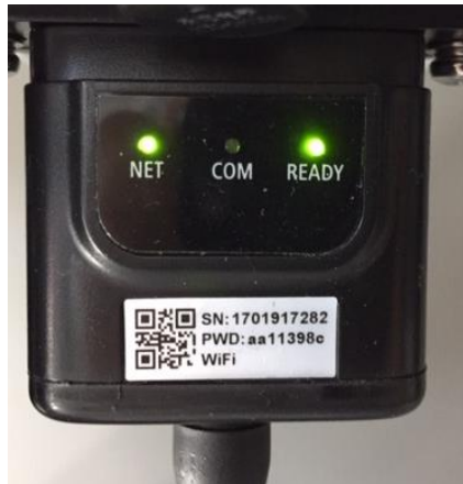
Figure 79 - Irregular communication status between inverter and Wi-Fi
