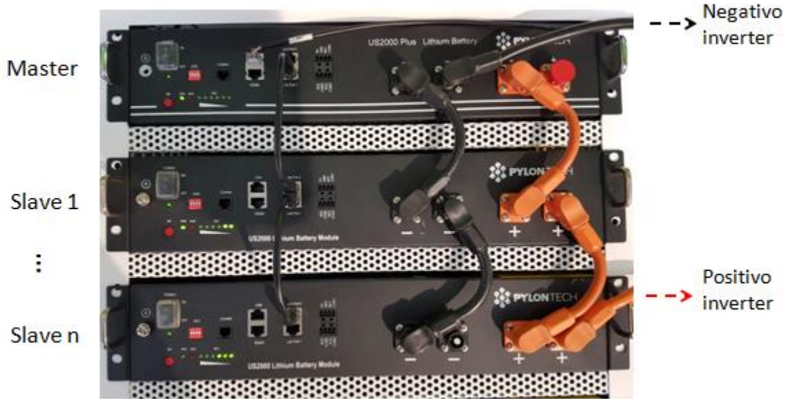
Figure 10 - Connecting three Pylontech batteries in parallel
