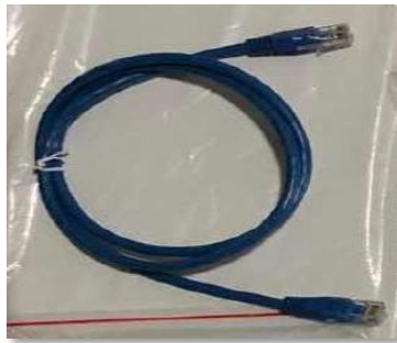
Figure 14 - Communication cable between WeCo 4k4 batteries
