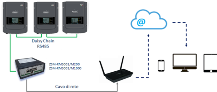
Figure 99 – Diagram showing the operation of the ZSM-RMS001/M200 / ZSM-RMS001/M1000 datalogger
