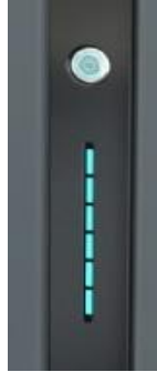
Figure 41 - POWER button of the AZZURRO 5000 battery
