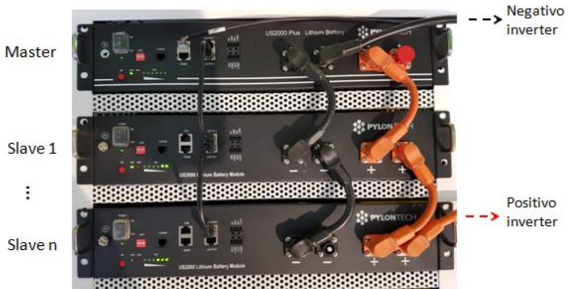
Figure 10 - Connecting three Pylontech batteries in parallel
