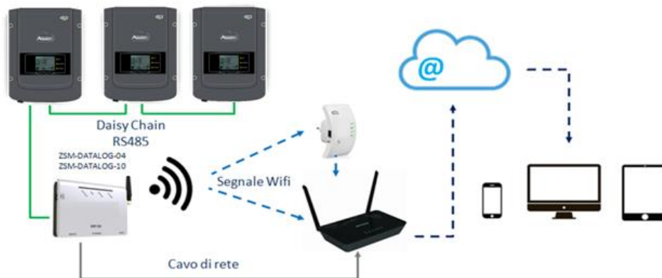
Figure 112 – Diagram for connecting the ZSM-DATALOG-04 / ZSM-DATALOG-10 datalogger
