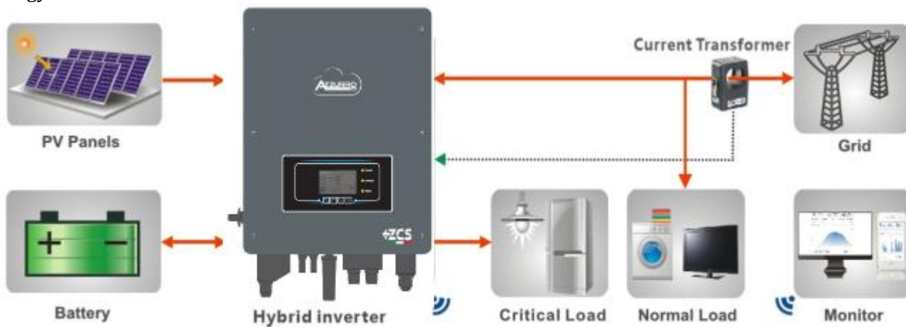
Figure 1 - Diagram of a system on which an 1PH HYD3000-HYD6000-ZSS hybrid is installed
