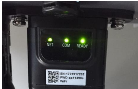
Figure 109 - Final status of LEDs
