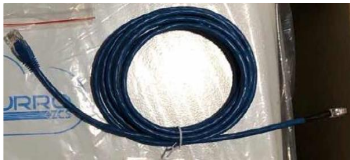
Figure 26 - Communication cable between the inverter and WeCo 5k3 battery
