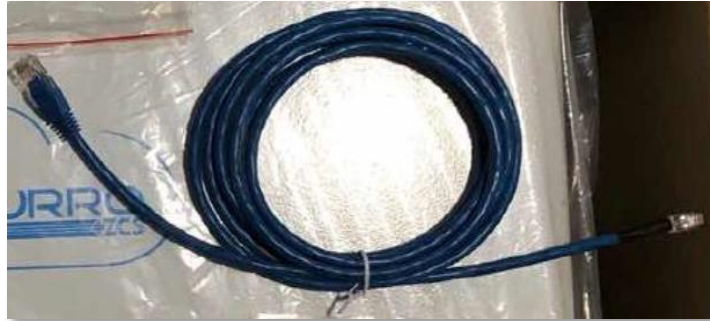
Figure 12 - Communication cable between the inverter and the WeCo PRO 4k4 battery
