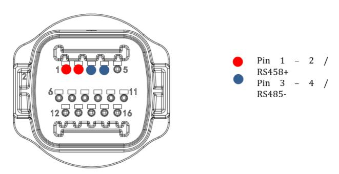
Figure 98b - Connecting the serial line via the communication connector for 1PH 3000-6000 TLM-V3, 3PH HYD5000-HYD20000-ZSS
