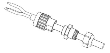
Figure 19 - Connecting the AC output cables (2)
