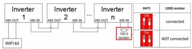
Figure 83 - Positioning of dip switches to connect the isolation resistor
