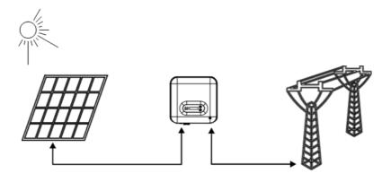
Figure 2 – Grid-connected photovoltaic system
