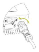
Figure 22 - Disconnecting the AC output cables
