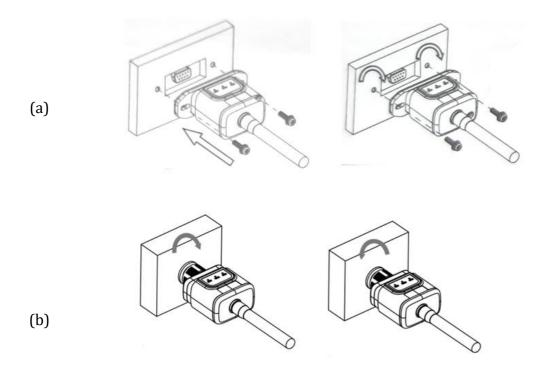
Figure 39 - Inserting and securing the external Wi-Fi adapter
