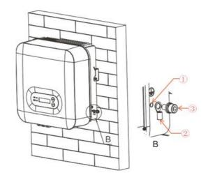
Figure 18 - Inverter external grounding instruction diagram
