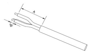
Figure 18 - Connecting the AC output cables (1)
