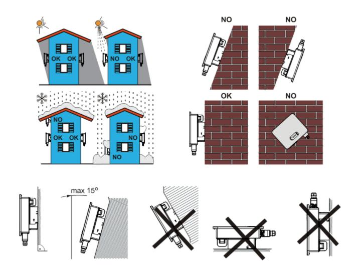
Figure 4 - Requirements or installing a single inverter
