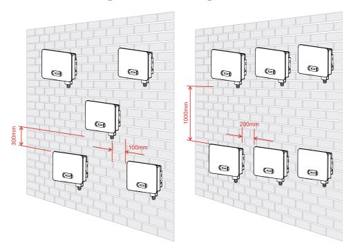
Figure 11 - Clearance for multiple inverters
