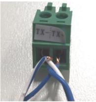
Figure 80 - Tightening the network cable to the RS485 terminal block
