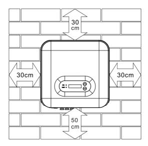
Figure 10 - Clearance for single inverter
