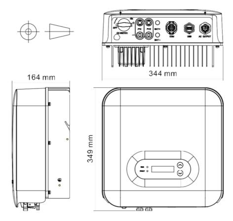
Figure 3 - Front and side view of the inverter
