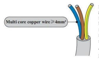
The cross-section of the power line must be sized in order to prevent unwanted disconnections of the inverter from the grid due to high impedance of the cable connecting the inverter to the point of supply. In addition, the AC cable must be correctly sized to ensure that the loss of power on the cable is less than 1% of the rated power and to ensure the proper functioning of the anti-islanding protection. The cable length from the inverter to the grid should not exceed 100 metres.
