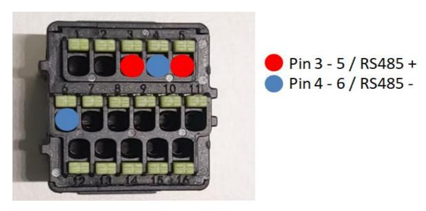
Figure 98c - Connecting the serial line via the communication connector for 1PH HYD3000-HYD6000-HP
