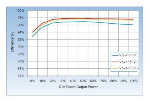
Figure 7 - Power efficiency curve
