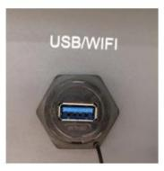
Figure 38 - Port for external Wi-Fi adapter
