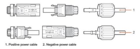
Figure 14 - Connecting the DC input power cables (2)
