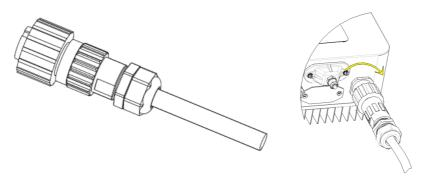
Figure 21 - Connecting the AC output cables (4)
