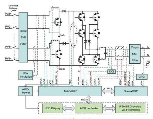
Figure 6 - Schematic diagram
