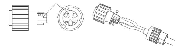
Figure 20 - Connecting the AC output cables (3)
